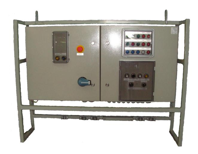
Switchgear BTW - 05/7 is an electrical device designed for use in underground mining in non-explosive hazard conditions as well as on the ground. Switchgear type BTW - 05/7 is designed to connecting and switching on air regulating damper (with AUMA NORM drives), controlling the flow of air through gangways, in a 3-phase mine grid with isolated star point of the transformer (IT) for rated grid voltage of 500V.
